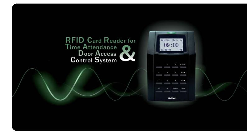
Kadex, a time attendance & door access control RFID card reader supports RFID card ID, 5-digit password or combination of both. Kadex terminal works with security alarm system to alert users in cases of break in and when duress function in Kadex reader is used. The terminal can integrate with fire alarm system to unlock all doors when fire alarm is triggered.
